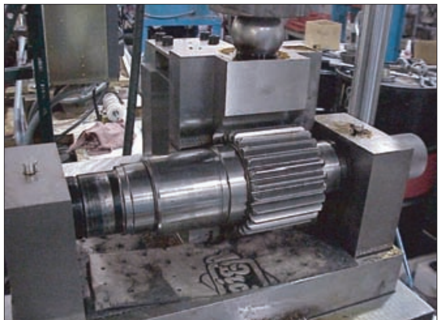
Single-tooth bending fatigue test on a helicopter main transmission gear is performed at the Gear Research Institute (courtesy Gear Research Institute).
