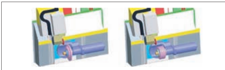
Figure 7—Grind head for profile and threaded wheel grinding.
