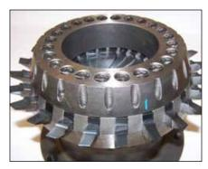
Gleason Corporation recently introduced Coniflex Plus, a high-speed dry cutting tool system for manufactur-
