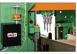
The Unist lubricator is a through-thetool MQL/near dry machining system that when used with the Coolube lubricant, eliminates the need for flood coolant and improves drill life.
