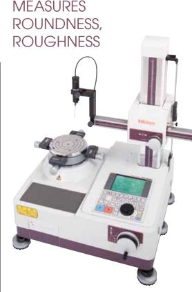
Two metrology products from Mitutoyo America Corporation were released: the Roundtest RA-220 roundness measuring machine and the Surftest SJ-210 portable surface roughness tester.
