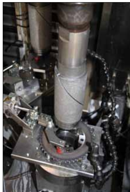
Each spindle removes about 0.025 mm from the bore.
