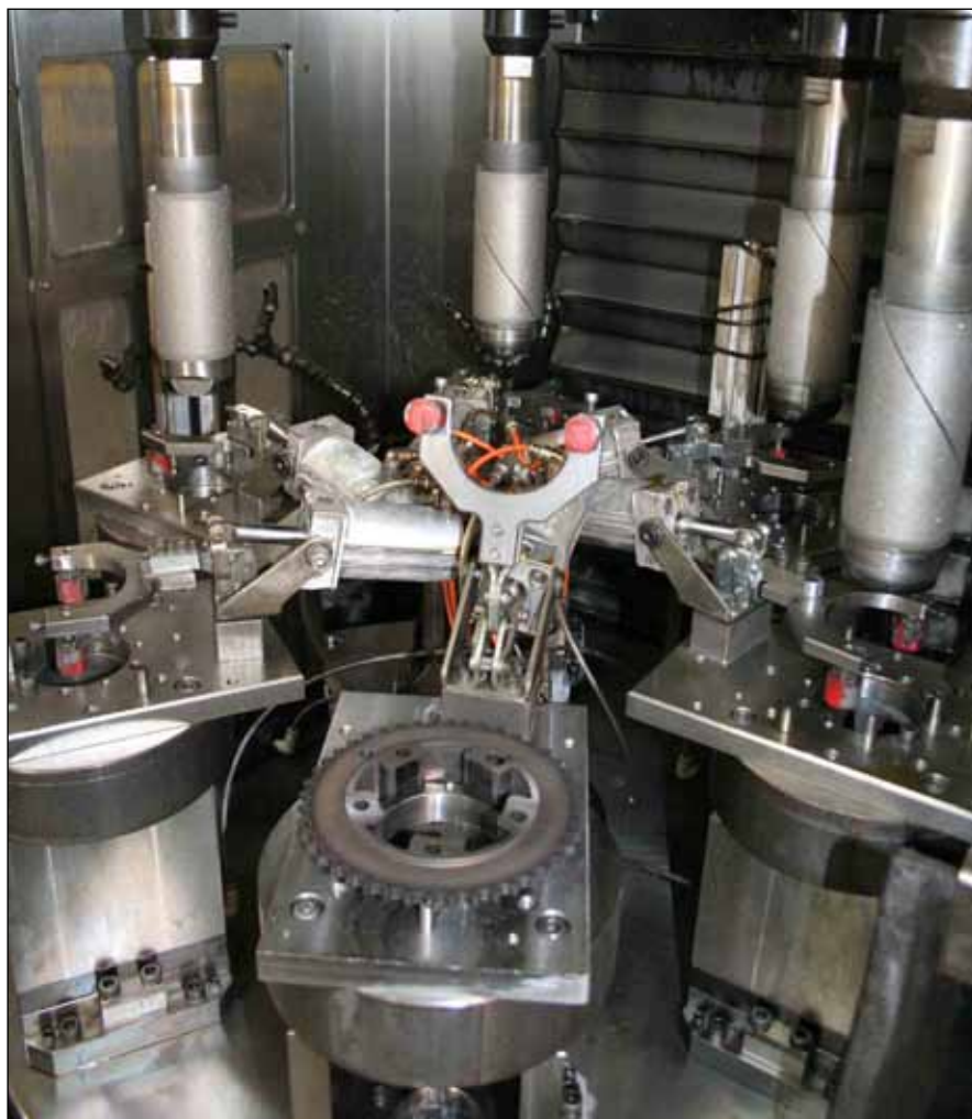
The honing system at Cloyes' Subiaco plant employs four spindles and an automated part load/unload system. VSS-2 machines can be equipped with up to six spindles.
