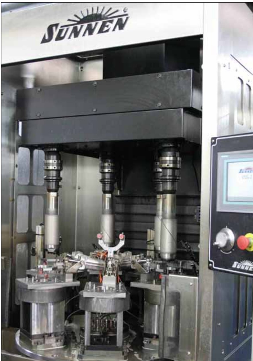
The VSS-2 Honing System from Sunnen helps Cloyes Gear maintain productivity and process capability in the manufacture of its variable valve timing stators.
