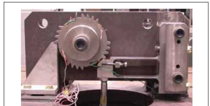
Figure 11—STBF test fixture with asymmetric gear installed.
