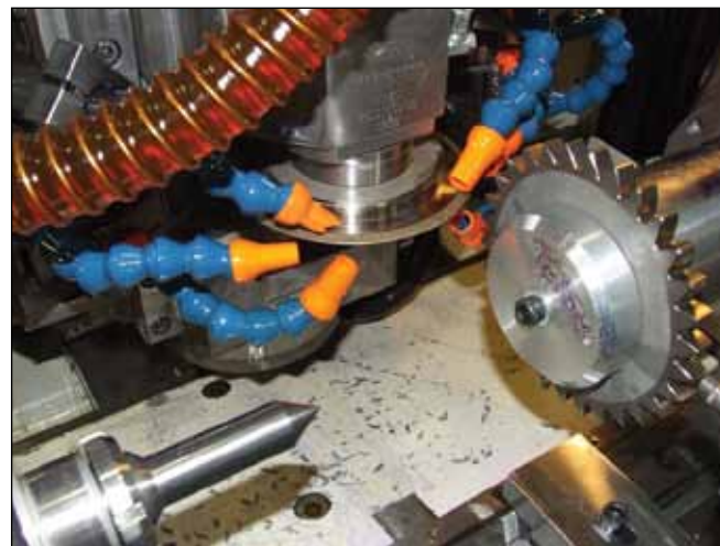
Figure 9—Gear form grinding set-up with CBN grinding wheel.
