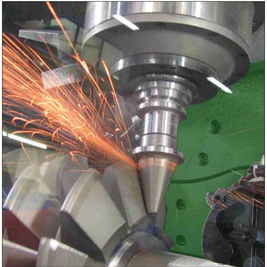
The Corvus CPP 1100 was created to meet the demand for large or coarse pitch hob manufacturing (courtesy of Schneberger).
