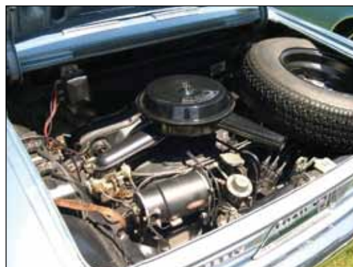
Photo of Chevrolet Corvair 164 Turbo rear-mounted engine—and spare tire compartment!—taken at Bay State Antique Automobile Club's July 10, 2005 show at the Endicott Estate in Dedham, MA (courtesy of User: Sfoskett/WikimediaCommons).
