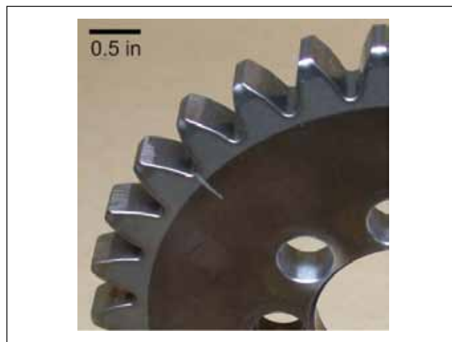
Figure 17—Scuffing failure of baseline test gear.
