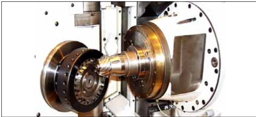
Figure 7—Hypoid pinion cutting with face hobbing cutter (continuous process).
