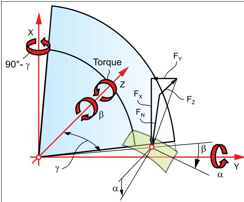
Figure 8—Force diagram for calculation of bearing loads.
