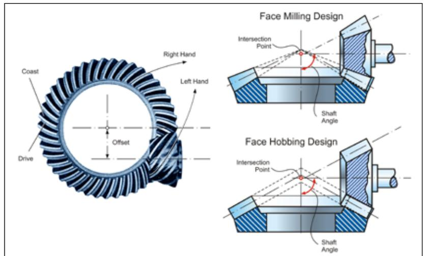
Figure 2—Hypoid gear geometry.
