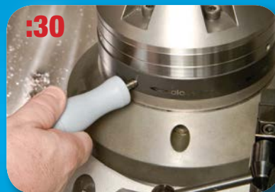
With just the twist of the activation handle installation is now complete.
