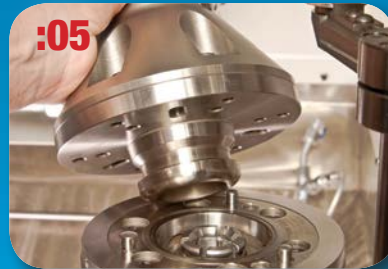
Install a new Quik-Flex®Plus module onto the common workholding interface...
