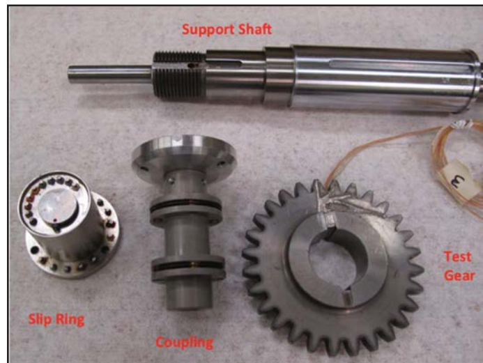
Figure 11 Loss-of-lubrication test specimen and related components.
