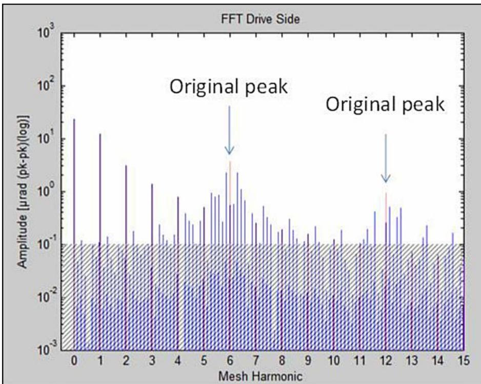
Figure 18 Comparison of FFT of transmission error, including introduced surface structure with (blue) and without (red, Fig. 7) shift of structure from flank to flank, leading to lowered peak harmonics and introduction of sidebands around 6th- and 12th-order mesh harmonics.
