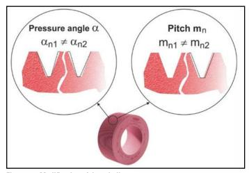
Figure 8 Modification of the grinding worm.
