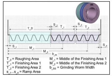
Figure 9 Grinding worm layout.
