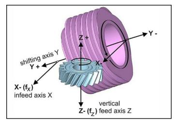
Figure 2 Continuous generating grinding principle.
