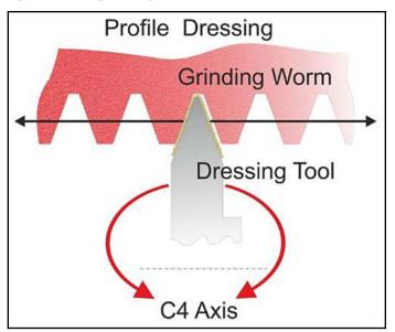
Figure 10 Dressing the grinding worm.
