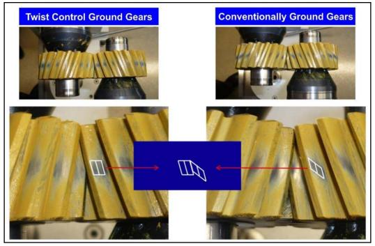
Figure 15 Contact patterns of mating gears.
