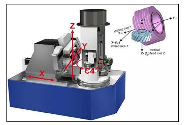
Figure 3 Machine axis movements.
