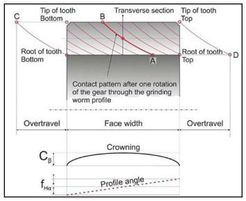
Figure 6 Crowning and profile angle.
