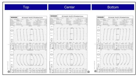
Figure 14 Mating gear ground with natural twist.
