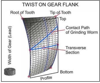
Figure 4 Flank twist.
