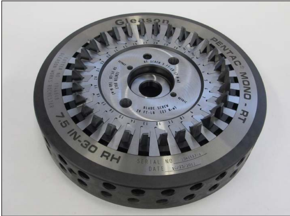
Figure 1 Face cutter head (Face Milling) with stick blades (Ref. 2).
