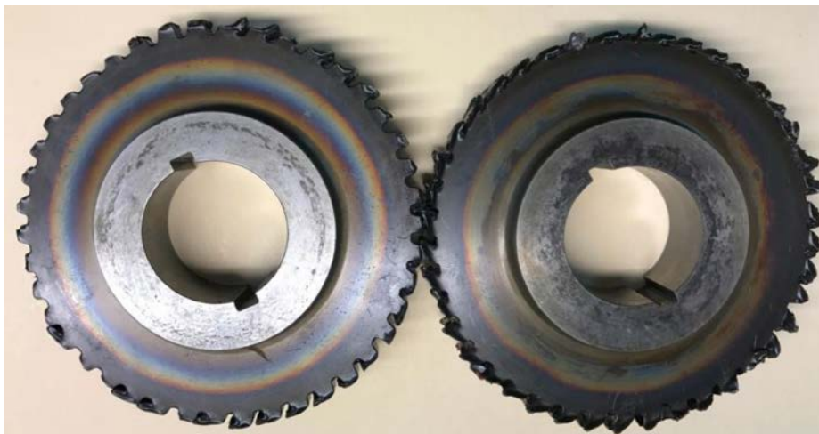
Figure 7 Catastrophic failure, run to loss of power transmission.
