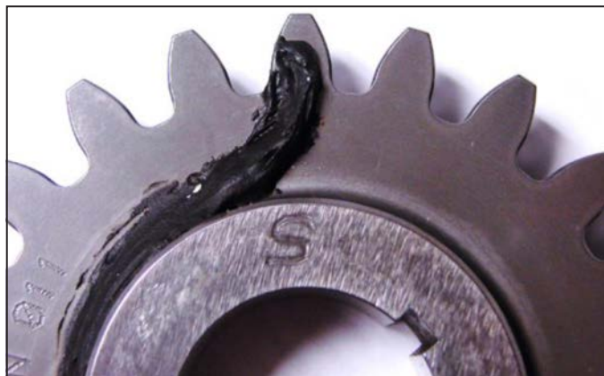
Figure 12 Thermocouple instrumented gear.
