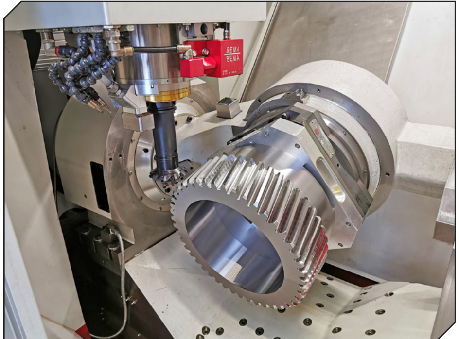
High-quality gearwheels are produced from hardened blanks within a very short time on 5-axis milling centres supplied by Röders.
