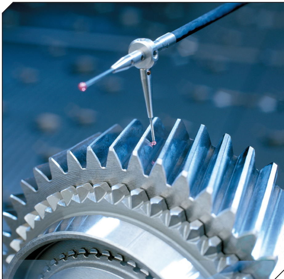
Depending on the probe-type, a CMM can provide a wide range of gear measurements, including gear-tooth profiles, faster than dedicated gear measurement machines while delivering needed accuracy.
