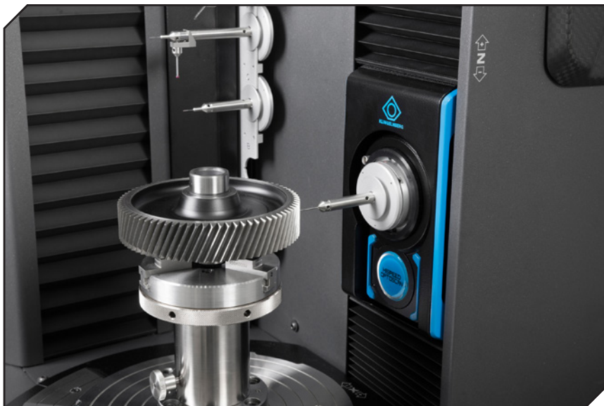
Profile and lead trace measurement with tactile NANOSCAN sensor.
