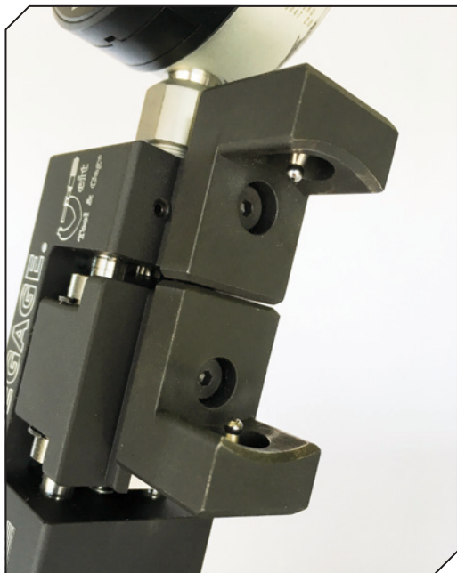
Figure 2 ONEGAGE tooling with integral balls for measuring external pitch diameter.
