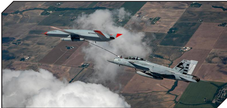
The MQ-25 T1 test asset refuels a Navy F/A-18 during a flight June 4 at MidAmerica Airport in Illinois.
