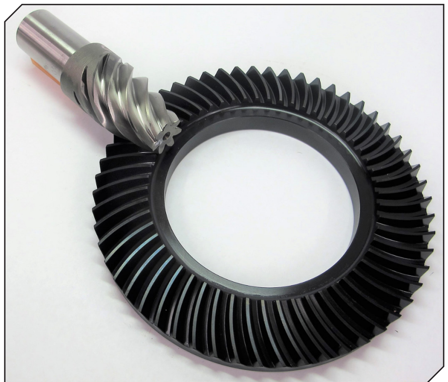
Figure 2 Hypoid gearset with a ratio of 7 × 55.
