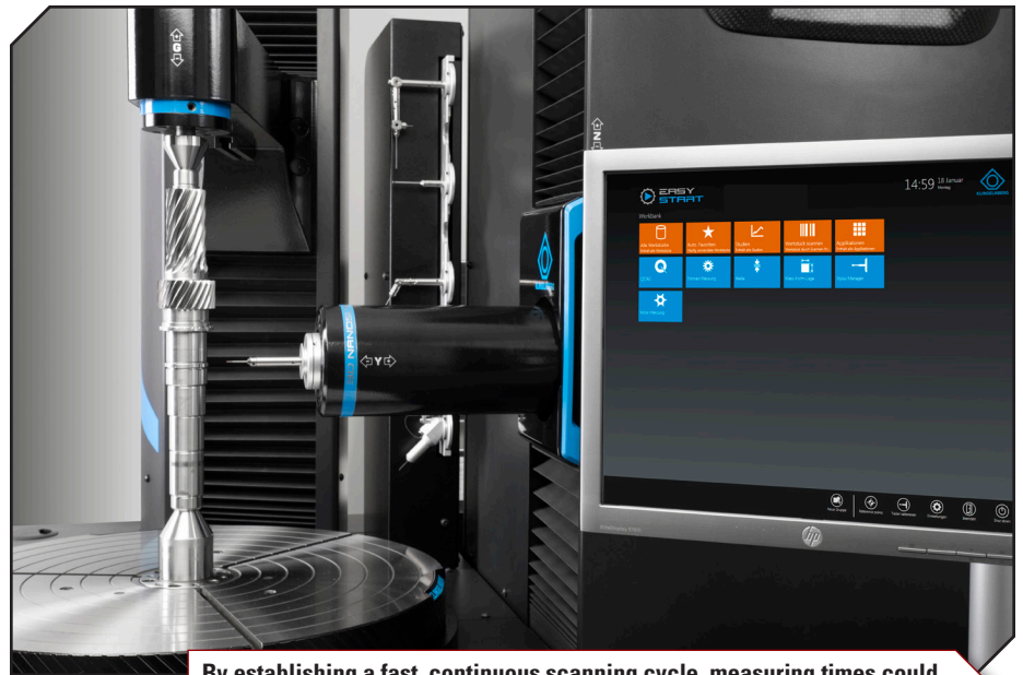
By establishing a fast, continuous scanning cycle, measuring times could be reduced by nearly 50% without compromising on accuracy.
