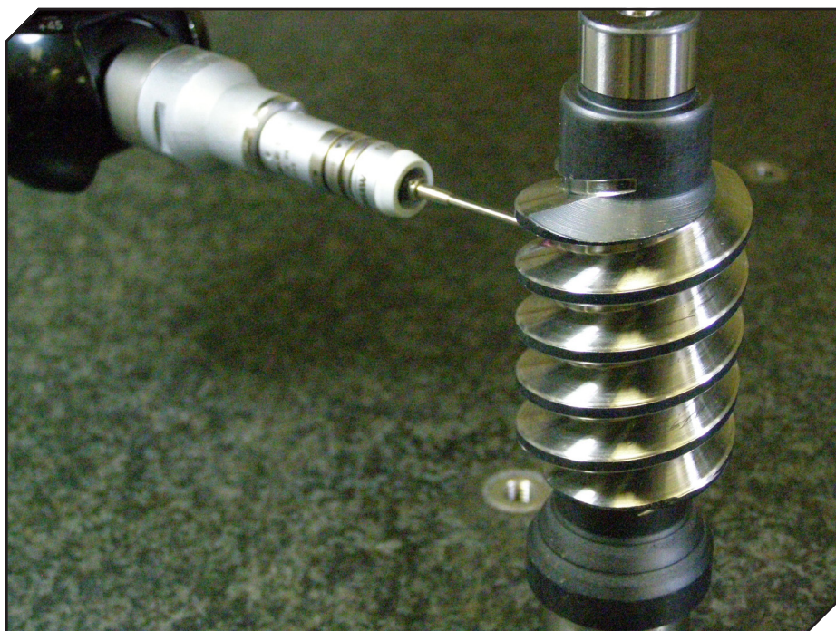
A CMM can measure many different types and sizes of gears such as the worm gear pictured.
