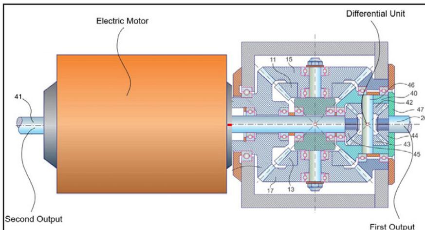
Figure 6 Double differential between the driving wheels—Solution 1..
