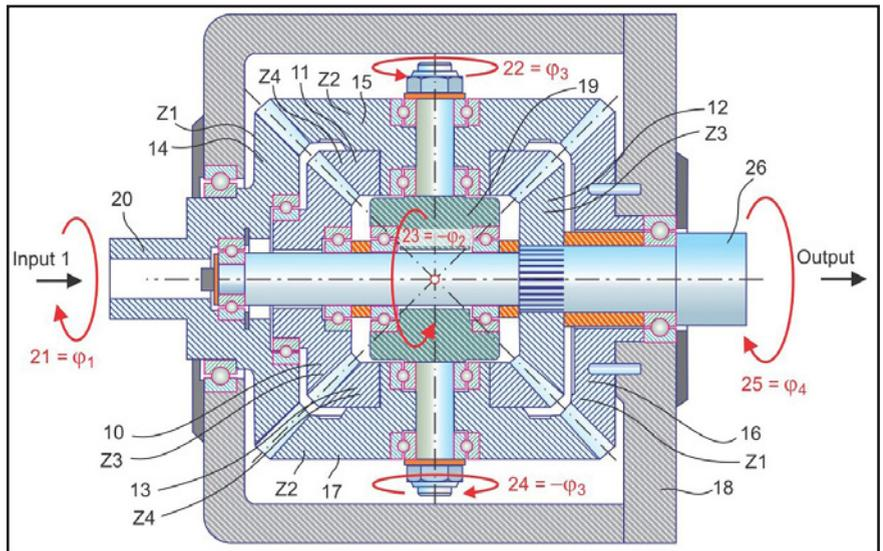
Figure 2 Double differential transmission.
