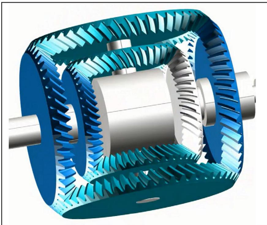
**Figure 8** KISSsoft animation—Double differential with ratio 18.
