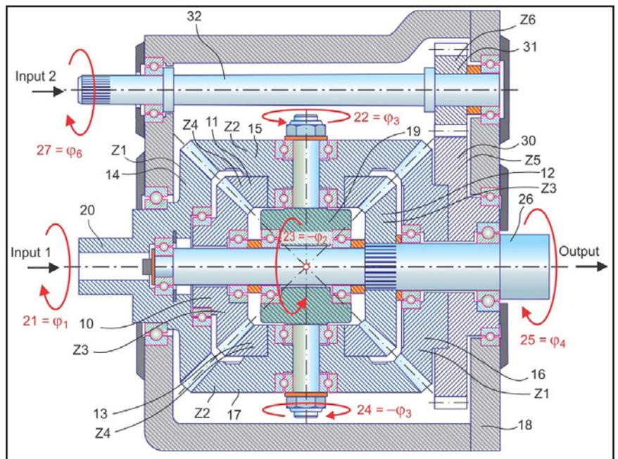
Figure 3 Extended double differential with two inputs.
