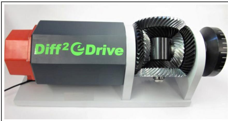
**Figure 9** Prototype transmission with motor—Ratio 81.
