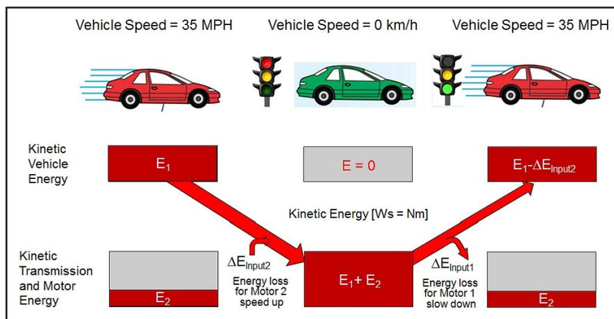
Figure 4 Energy balance—vehicle with mechanical energy storage.
