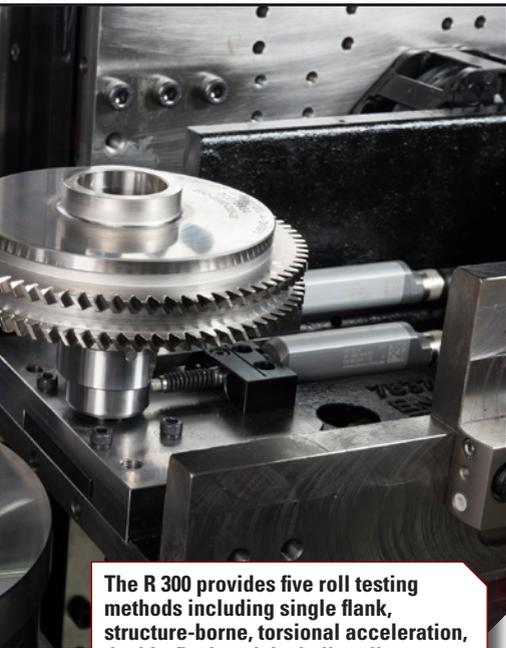
The R 300 provides five roll testing methods including single flank, structure-borne, torsional acceleration, double-flank and the helix roll test. (Courtesy Klingelberg)
