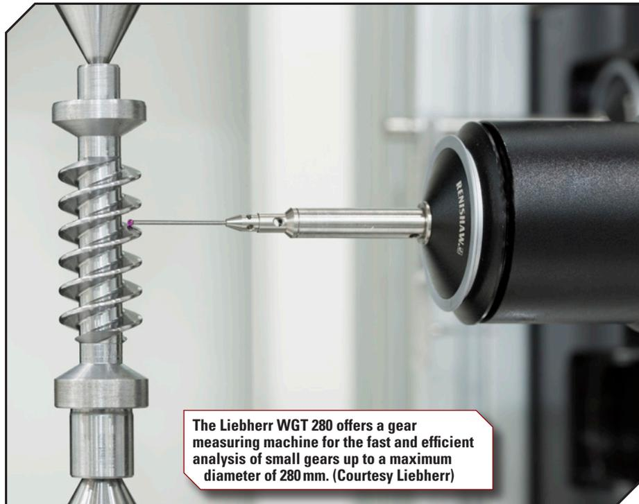
**The Liebherr WGT 280 offers a gear measuring machine for the fast and efficient analysis of small gears up to a maximum diameter of 280 mm. (Courtesy Liebherr)**
