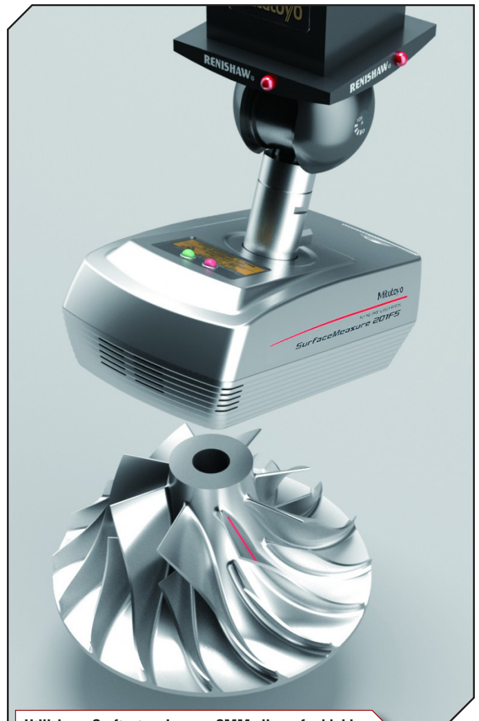
Utilizing a Surftest probe on a CMM allows for highly accurate measurements of complex parts, including gears and impellers.
