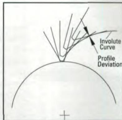
Fig. 6—Profile deviation from the ideal involute made by a hob with more gashes.
