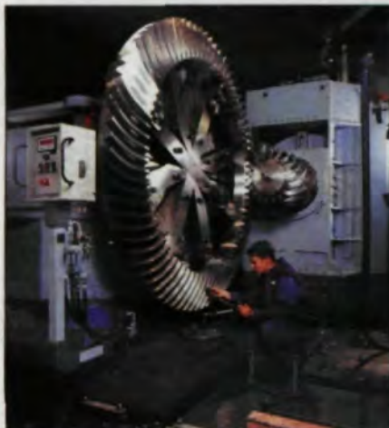
An ATA Gears employee kneels between the main parts of a specially modified machine that finish-machines and single-flank tests large spiral bevel gear sets.
