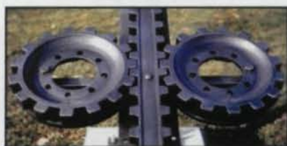
A segment of the Pilatusbahn's rack and cogwheel assembly is displayed as an outdoor sculpture at Alpnachstad, the railway's station at the foot of Mount Pilatus. (Photo courtesy of ASME International.)
