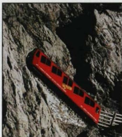
The Pilatusbahn is a cogwheel railway in Switzerland and climbs 1,689 vertical meters to the top of Mount Pilatus. The steep climb has a maximum grade of 48 percent, or 21.6 degrees.
