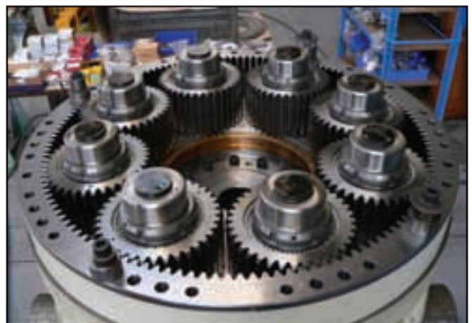
Orbital2's gearboxes for the one-megawatt prototype feature eight planetary spur gears in the first-stage transmission, with four planetary spurs in the second stage, followed by a parallel shaft output stage.
