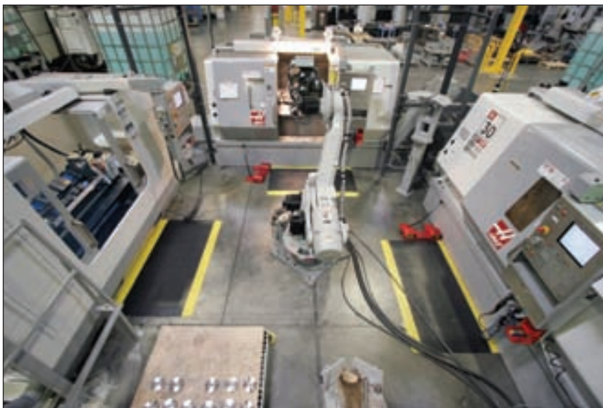
A Motoman 6-axis robot works between three Haas machines.
