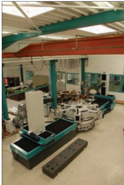
Wenzel’s dual arm gear measuring machine was designed to measure big gears (courtesy of Wenzel).
