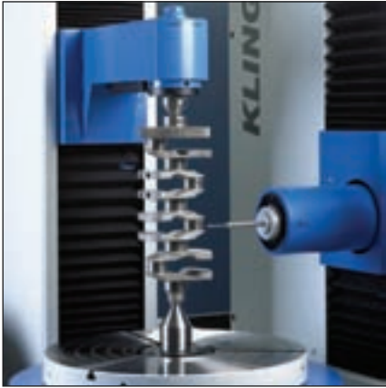
Crankshaft inspection from Klingelberg allows accurate dimension, form and position measurements (courtesy of Klingelberg).
