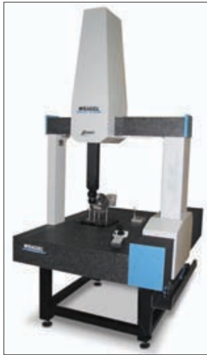
In the past, CMMs have been perceived as not being accurate enough for gears, but advances in software and laser scanning probes has changed this (courtesy of Wenzel).
