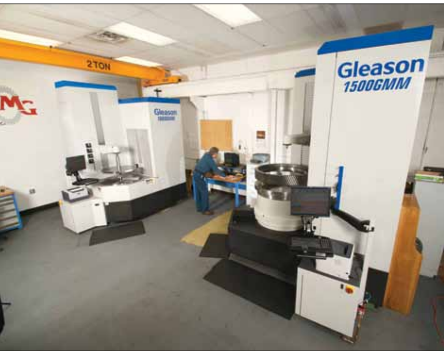
The QC lab at Milwaukee Gear was recently retooled with two large-diameter GMM inspection systems from Gleason.
