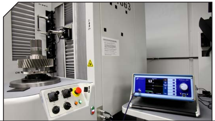
American Stress Technologies’ Rollscan 300 digital Barkhausen noise analyzer and probe are easily integrated into the Gleason 350GMS. End result? All of the necessary gear inspection can be conducted on a single GMS machine, in a single setup, saving time and helping ensure inspection accuracy.
