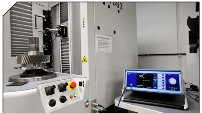
American Stress Technologies’ Rollscan 300 digital Barkhausen noise analyzer and probe are easily integrated into the Gleason 350GMS. End result? All of the necessary gear inspection can be conducted on a single GMS machine, in a single setup, saving time and helping ensure inspection accuracy.
