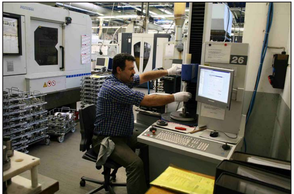
Figure 1 Gear inspection in a shop floor environment.
