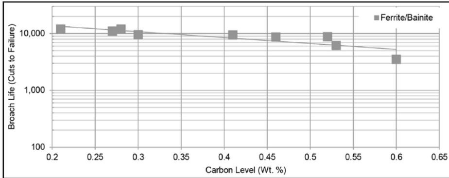
**Figure 7** Effect of carbon level on broach life of steels composed of ferrite/bainite structure.
