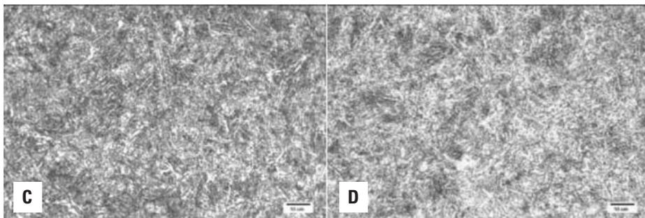
**Figure 11 Photomicrographs of 5046 bainite/martensite/ferrite conditions after tempering at a) 1,150°F; b) 1,200°F; c) 1,275°F; and d) 1,325°F, nital etch.**
