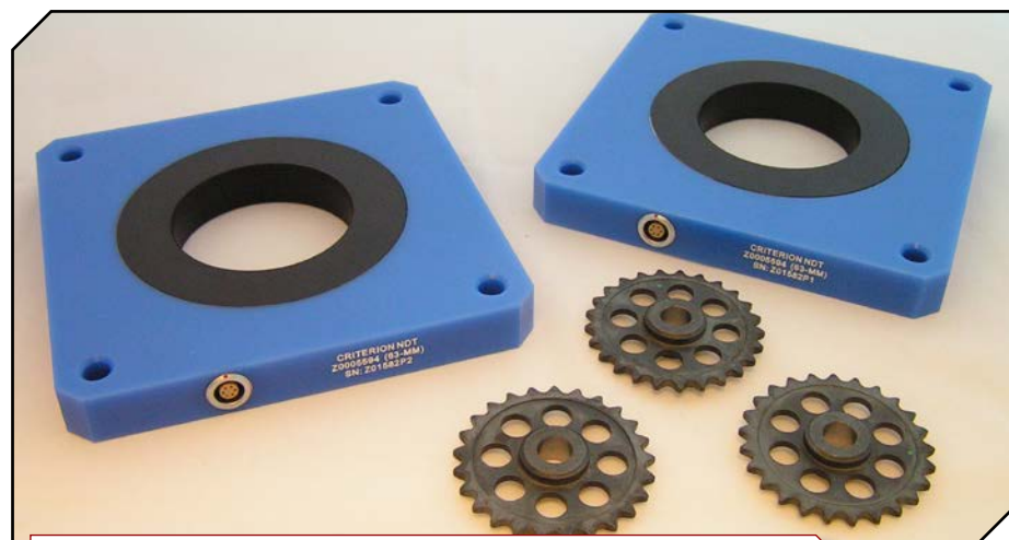
Gears and test coils that were part of an automated water pump assembly station. Eddy current test instrumentation and coils then confirmed heat treatment in advance of pressing the gears onto the water pump shaft.
