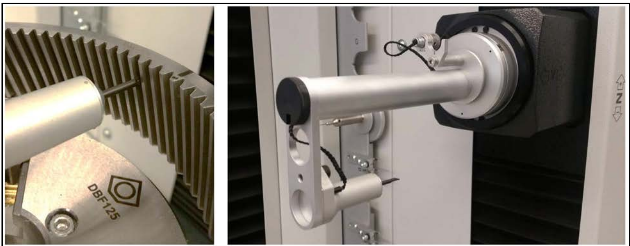
Figure 3 Roughness measurement—internal gears.
