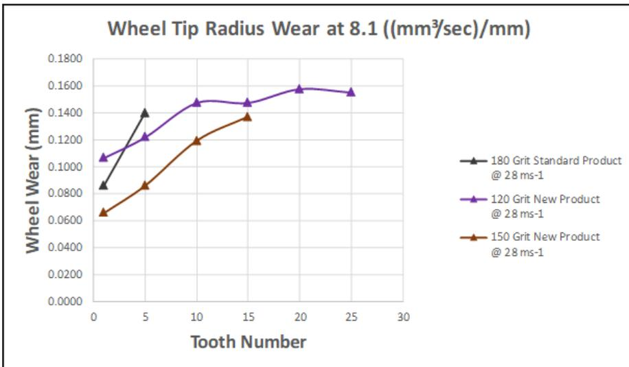
Figure 6 Wheel Tip Radius Wear for 8.1 MRR' at 28 ms<sup>-1</sup>.
