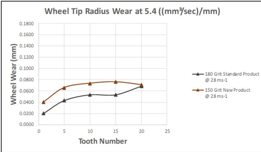
Figure 5 Wheel Tip Radius Wear for 5.4 MRR' at 28 ms<sup>-1</sup>.
