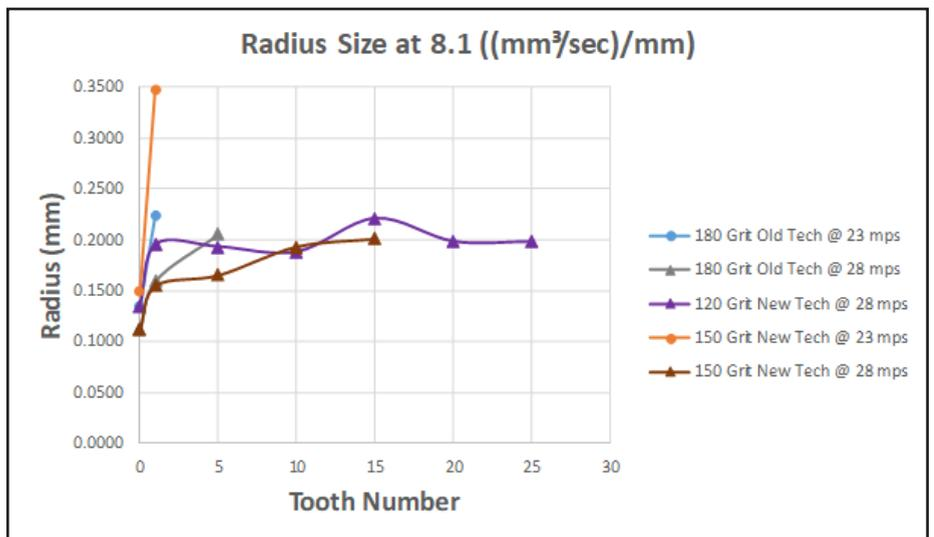
**Figure 4 Radius Size 23 ms<sup>-1</sup> vs 28 ms<sup>-1</sup>.**
