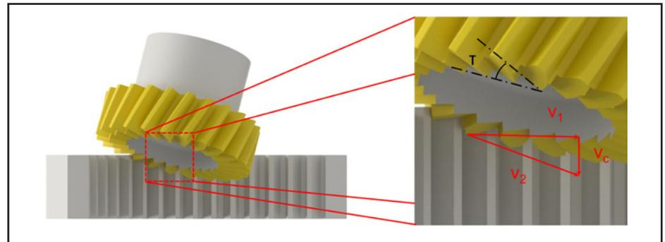
Figure 2 Cutting velocities during gear skiving ( $v_1$  rotation of the work gear,  $v_2$  rotation of the tool,  $v_c$  resulting cutting speed).
