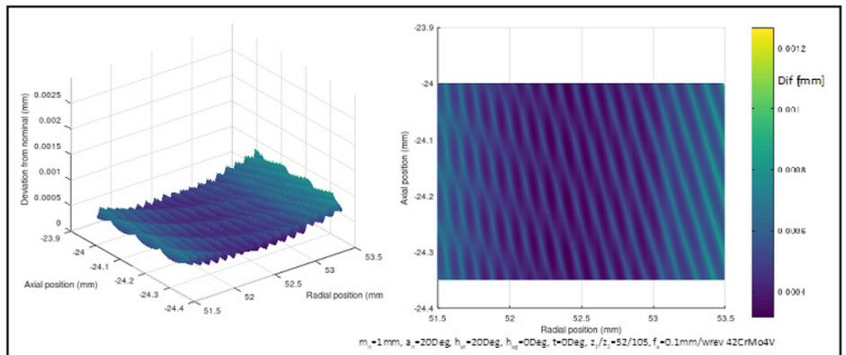
Figure 6 Work gear topography deviation 3D view (left) and top view (right).
