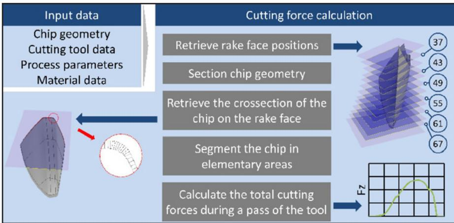
Figure 4 Cutting force calculation algorithm.
