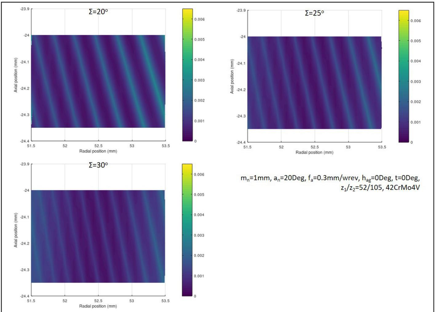
Figure 8 Influence of inclination angle on the gear topography.
