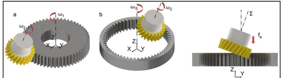
Figure 1 Gear skiving process kinematics for internal (b) and external gears (a).
