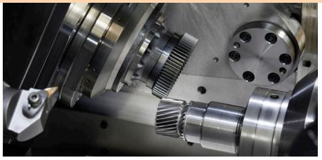
Figure 3—Skiving with running gear on an e-shaft. (Source: Pittler T&S)
