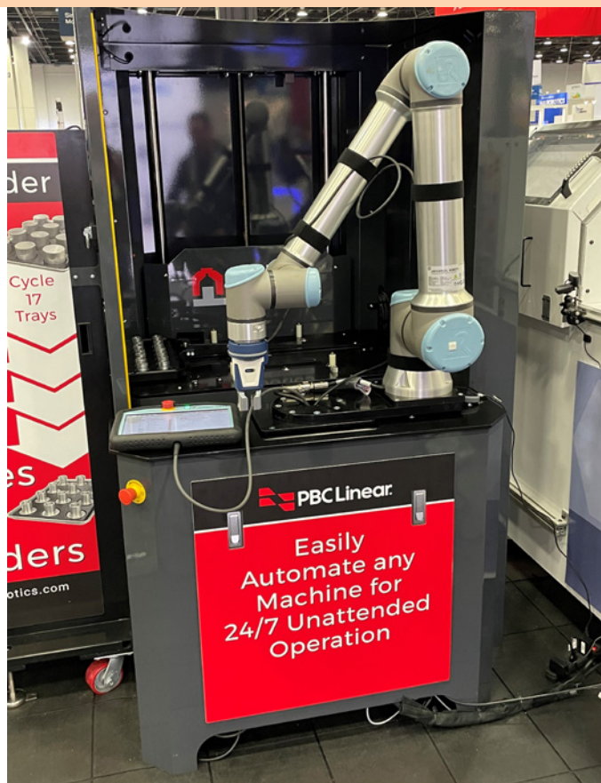
The Cobot Feeder from PBC Linear provides a platform for storing, staging, and safely delivering parts.
