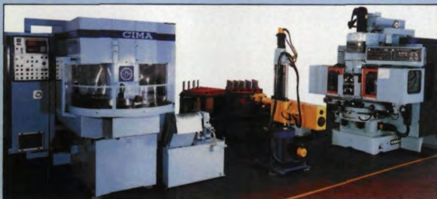
Robot Loading System
