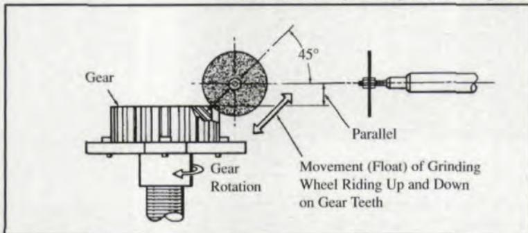
Fig. 4 — Alignment of grinding wheel.
