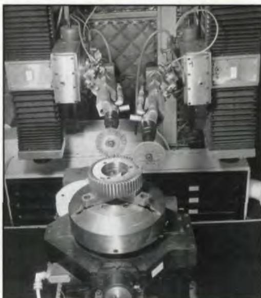
Fig. 2 — Deburring a spur gear with a brush followed by a grinding wheel.
