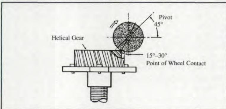
Fig. 6 — Helical gear wheel contact.
