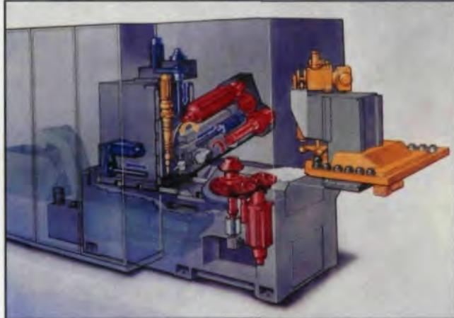
**Fig. 1 — Concept hobbing machine for dry hobbing. Courtesy of Liebherr America. Used with permission.**
