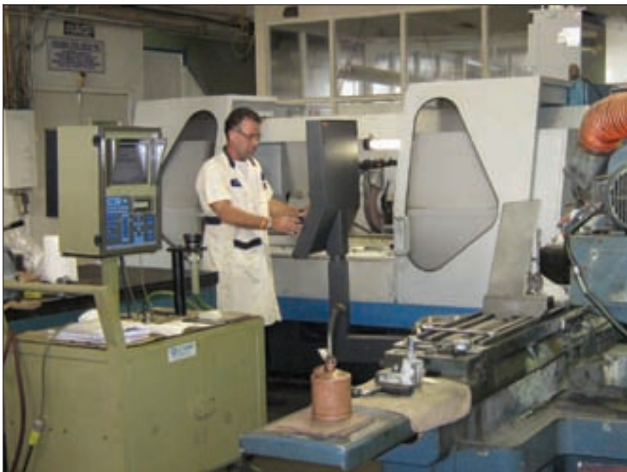
Colonial has put two conventional universal grinders and one CNC universal grinder in the same work area as a lean initiative. A jib crane was added for ease of handling (courtesy of Colonial Tool Group).
