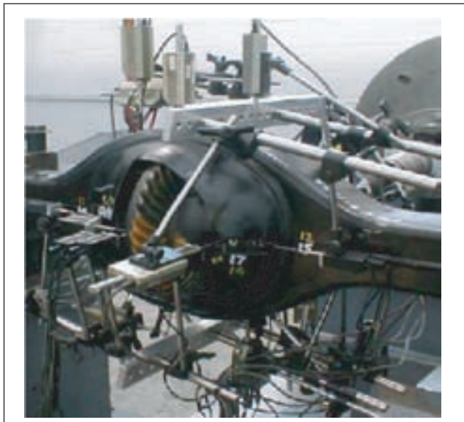
Figure 3—Experimental measurement of an axle deflection.
