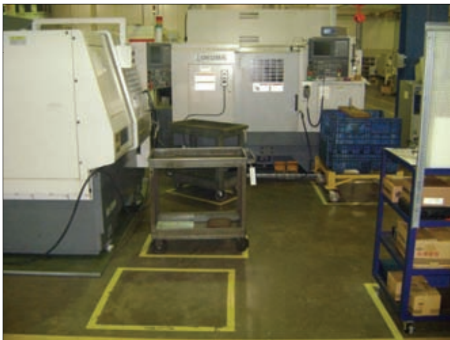
One of Schafer's many manufacturing cells are marked on the floor to maintain lean guidelines throughout the shop (courtesy of Schafer Gear).
