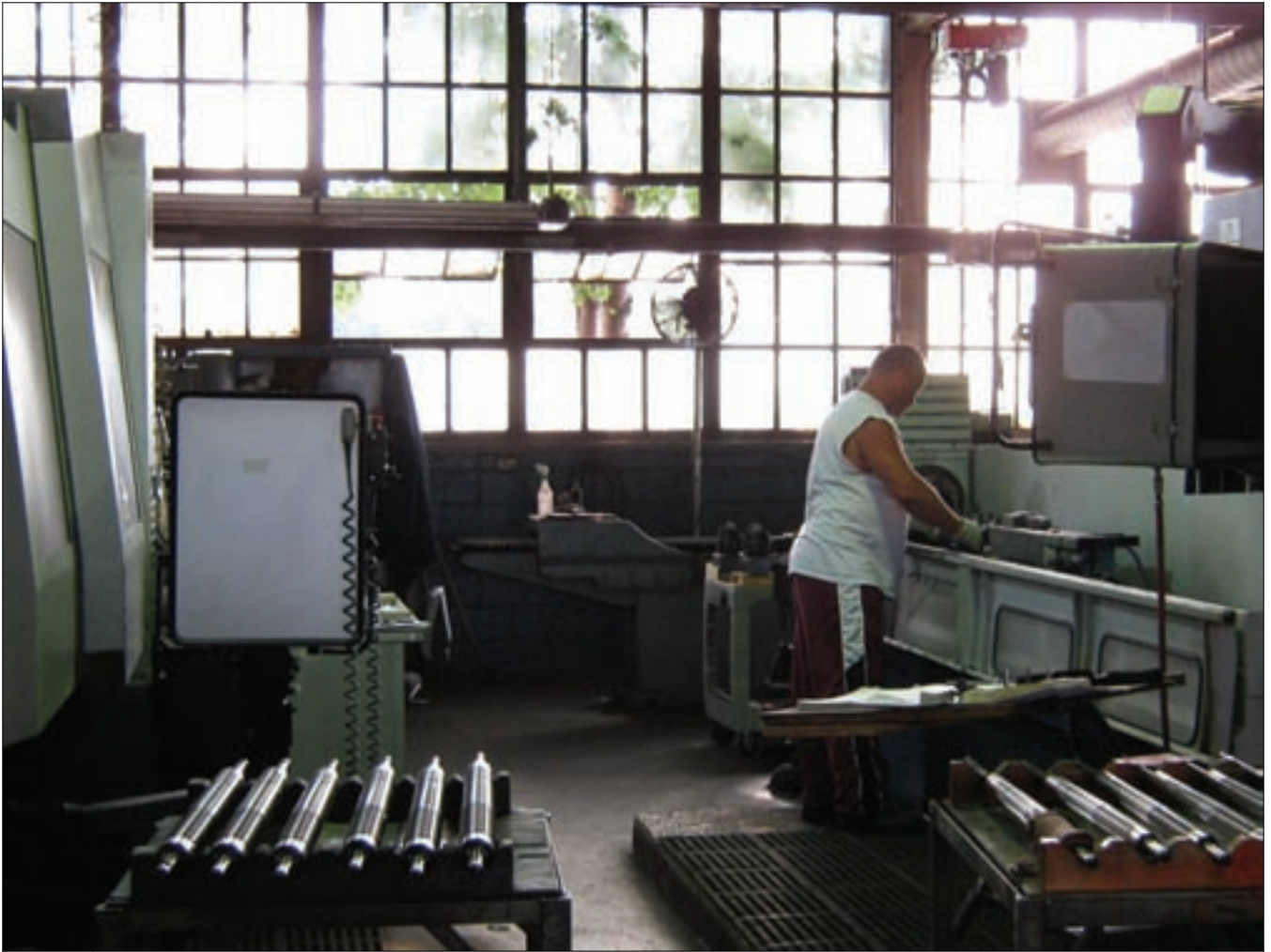
Thanks to lean principles, an operator in Colonial's spline department can run three machines at once, including two CNC spline grinders and a manual grinder (courtesy of Colonial Tool Group).
