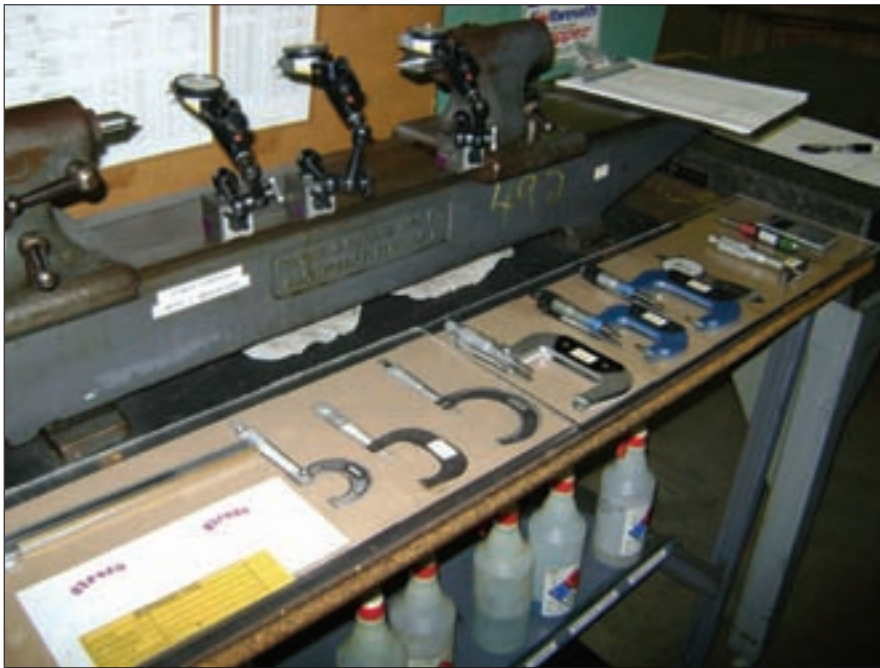
Schafer Gear demonstrates how the 5S strategy keeps its work stations organized and efficient. The gages missing at this station have a replica photograph under the plexiglass (courtesy of Schafer Gear).
