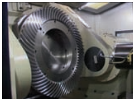
The HU80A-5X horizontal machining center cuts gears up to 35 inches by mounting the gear flat and then turning it up in an angle, so the end mills can cut at the best attitude to the gear profile.
