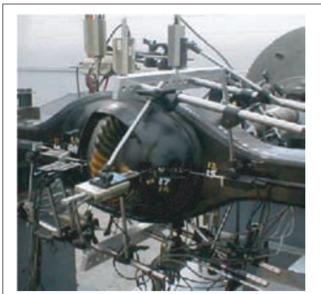
Figure 3—Experimental measurement of an axle deflection.
