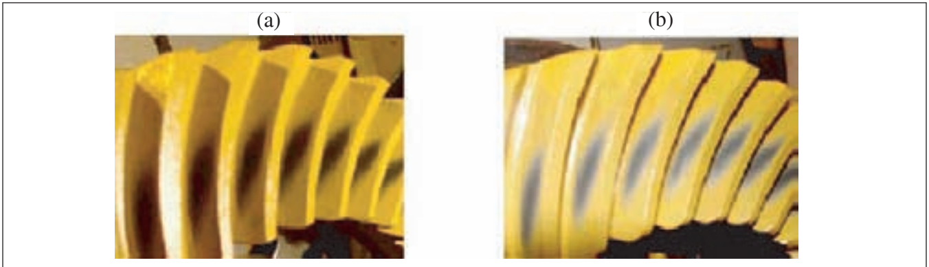
Figure 10—Representative contact patterns from samples of (a) Design 1; and (b) Design 2.
