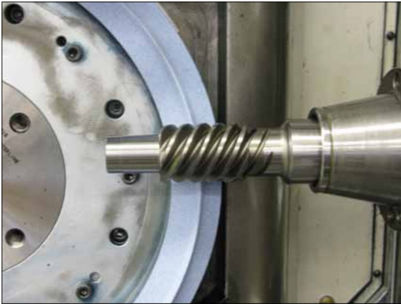
Figure 8—Super-reduction hypoid pinion grinding.
