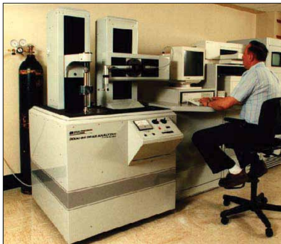
Gear measurement is an important step in troubleshooting the origins of gear noise (courtesy Penn State U).
