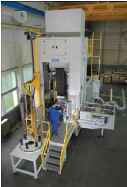
Advanced automation, material handling and CNC controls represent the latest in broaching technology. Pictured here is a 50-ton, two-station CNC helical broaching machine from Forst.
