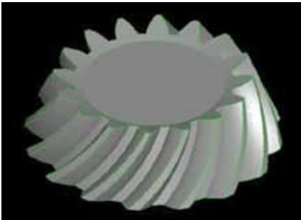
Figure 5—Tooth profile of pinion modeled using 3-D CAD system.
