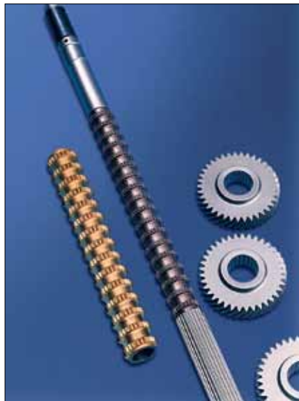
Hard broaching allows for cutting of hardened parts after heat treating. Shown here are hard broaching tools and sample parts. Courtesy of Forst Technologie GmbH.
