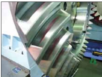
Figure 11—Tooth contact pattern of drive side.
