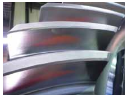
Figure 12—Tooth contact pattern of coast side.
