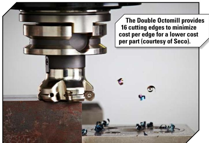
The Double Octomill provides 16 cutting edges to minimize cost per edge for a lower cost per part (courtesy of Seco).
