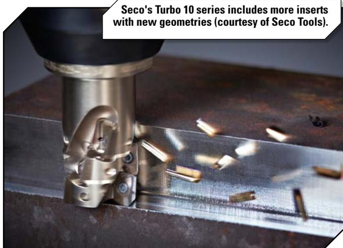
Seco's Turbo 10 series includes more inserts with new geometries (courtesy of Seco Tools).
