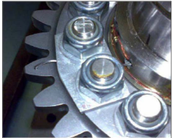
Figure 5 Gear equipped with thermocouple for bulk temperature measurement.
