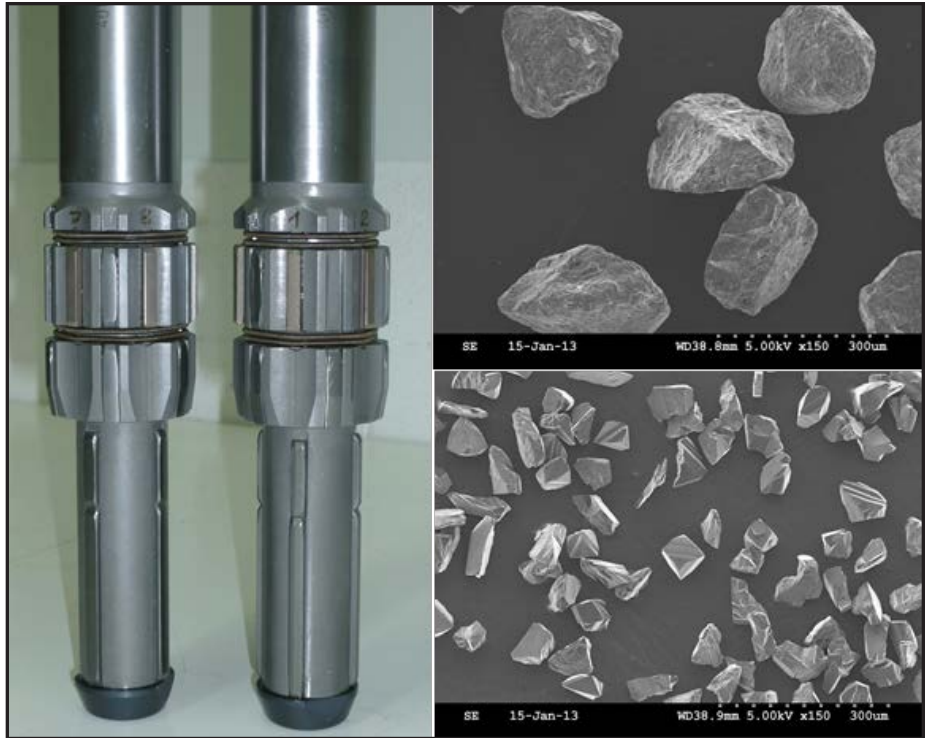
Figure 4 Hone tools with lower guides and CBN abrasive crystals (B213/B46).
