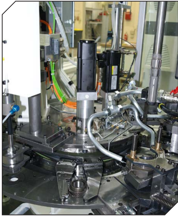
Figure 2 Machining stations for honing gear wheels.
