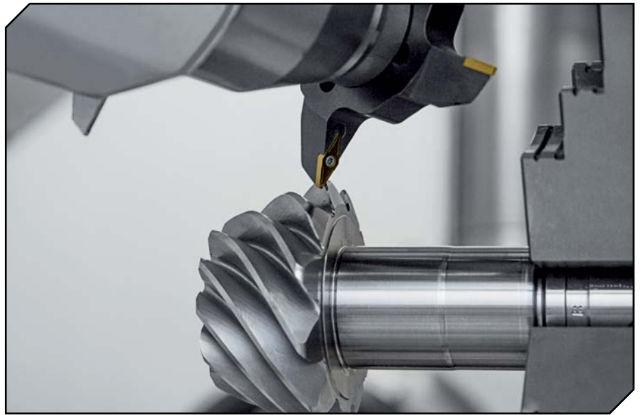
Autopath chamfering on a Gleason Phoenix 280CX, chamfer-cutting a bevel pinion.
