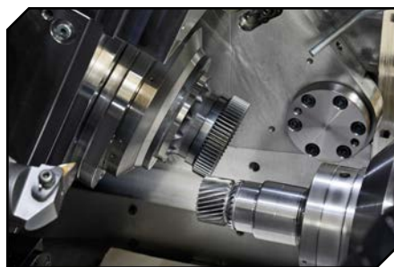
WMZ is demonstrating its Power Skiving gearing technology on an E-drive shaft.
