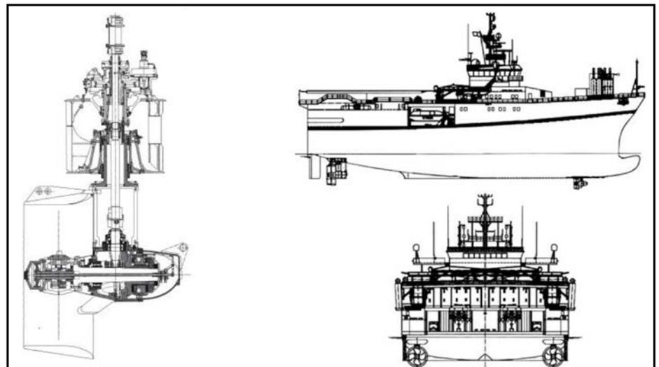
Figure 1 Positioning and design of the thruster (Ref. 16).
