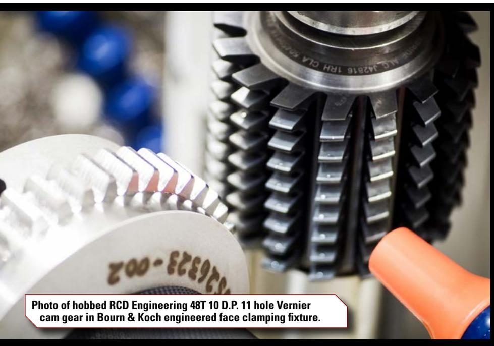
Photo of hobbed RCD Engineering 48T 10 D.P. 11 hole Vernier cam gear in Bourn & Koch engineered face clamping fixture.
