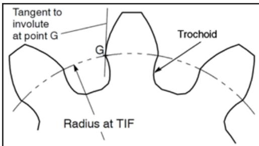
Figure 1 Root fillet shape of undercut teeth (Ref. 3).
