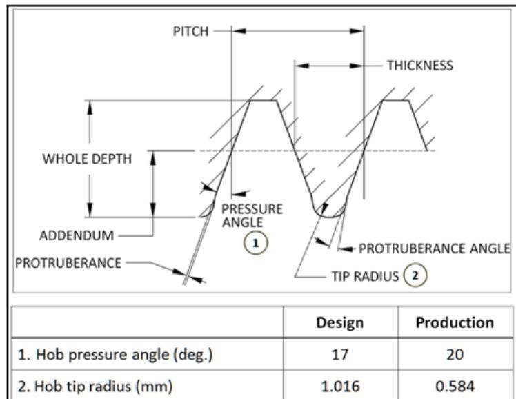
Figure 7 Comparison between design and production hob racks.
