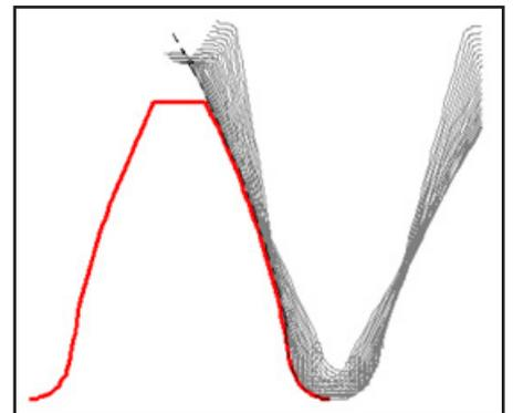
Figure 2 Gear tooth generated by a hob rack.
