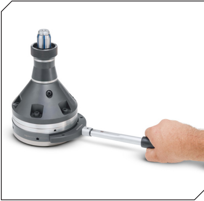
Gleason Quick-Flex Plus modular quick-change workholding system.
