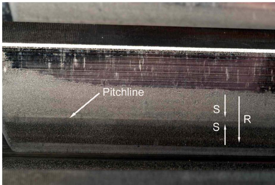
**Figure 2** The image shows a driven wind turbine pinion with micropitting. The pitchline is readily discernible because the floors of the micropit craters are oppositely directed in the addenda and dedenda, which resulted in light reflection directed into the camera lens in the addenda and directed away from the camera lens in the dedenda. This resulted in the addenda appearing light and the dedenda appearing dark.
