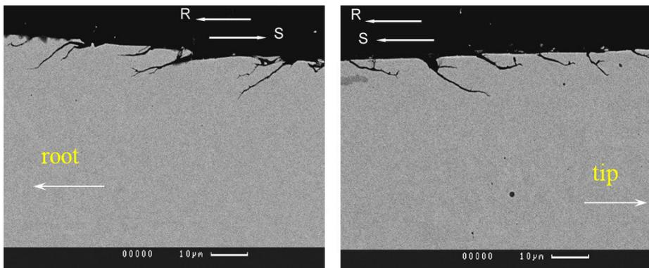
**Figure 1** The image shows two polished metallurgical specimens cut transversely through gear tooth micropitting. The left shows the dedendum, and the right shows the addendum of the tooth of a driven gear. The vectors R and S indicate the rolling and sliding directions. Micropitting cracks start at the gear tooth surface and grow at a shallow angle (typically 10–30 degrees, but sometimes as steep as 45 degrees) to the surface. Image courtesy of Newcastle University.
